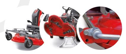
GSR+ Electric also enables **REAR DISCHARGE** option. This function can be obtained by simply removing a mulching plug placed under the mower deck, thanks to the operation of a conveniently placed lever on the right side (driver's side) of the mower's deck.
